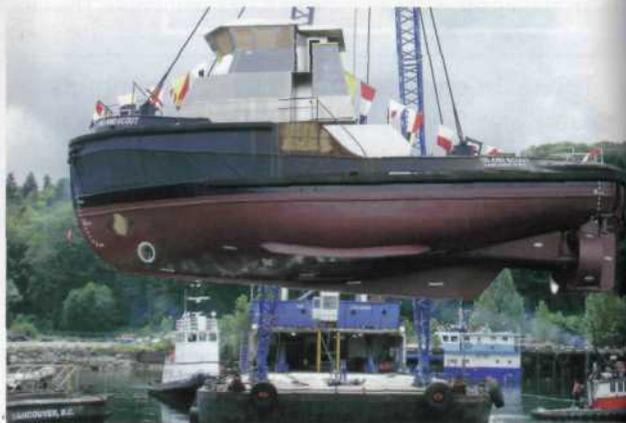
The **Island Scout** was launched into the water, less engines and machinery in July 2005. In this photo taken during the water launch, the tug's rounded moulded hull form is clearly visible.
