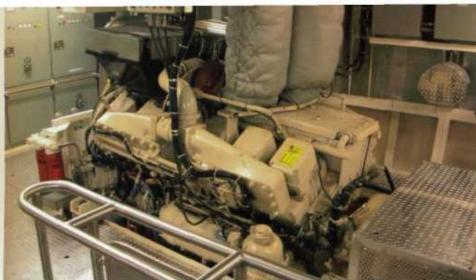
Power for the **Island Scout** is a pair of Cummins KTA38 M0 main engines with dual 800/500 horsepower ratings, linked by Centalink flexible coupling to Twin Disc MG 5222 gears with 6.10:1 reduction.
