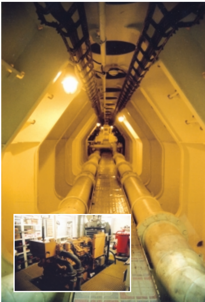
Two hydraulic motors feed into a common gearbox to power the Island Trader's omni-directional 700-horsepower Schottel SPJ 132 bow thruster.
