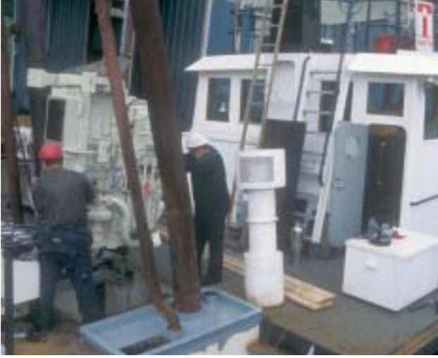
*Island Tug and Barge's maintenance crew lowers one the new Cummins diesels through a hatch in the top of the **Island Crown's** fiddle. The engines, lifted with a specially-designed jig, were stood on their head to fit through the hatch with mere inches to spare.*
